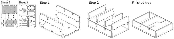
Tray 6 (the tray is higher on one side, make sure the long walls are correctly orientated)
